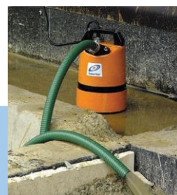
Puddle pump in use
